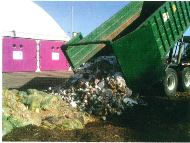
The pilot project is sized to process 5,000 tons/year of mixed food waste (70% of mix) and ground yard trimmings (30% of mix).
